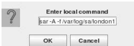
Figure 13-1. Executing a local command from kSar
